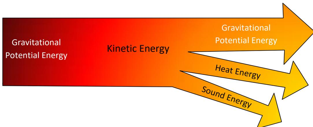
The reason that the cycle depicted in the above diagram does not continue indefinitely is because of the efficiency losses in the form of friction. Friction continuously leaks energy from the system in the form of heat and sound energy. This explains why the efficiency of each track is less than 100%.
