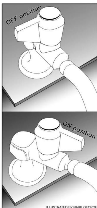
**Figure 2: The Bunsen burner tap in the open and closed positions**
