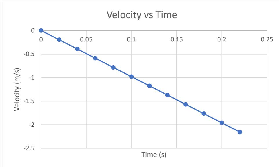
Figure 4 – The velocity vs time graph for the free fall
