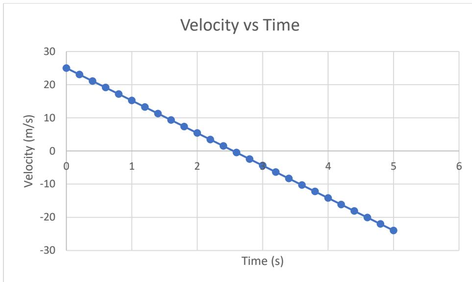
Figure 6 – Velocity vs time graph for a ball thrown upwards with an initial vertical velocity
