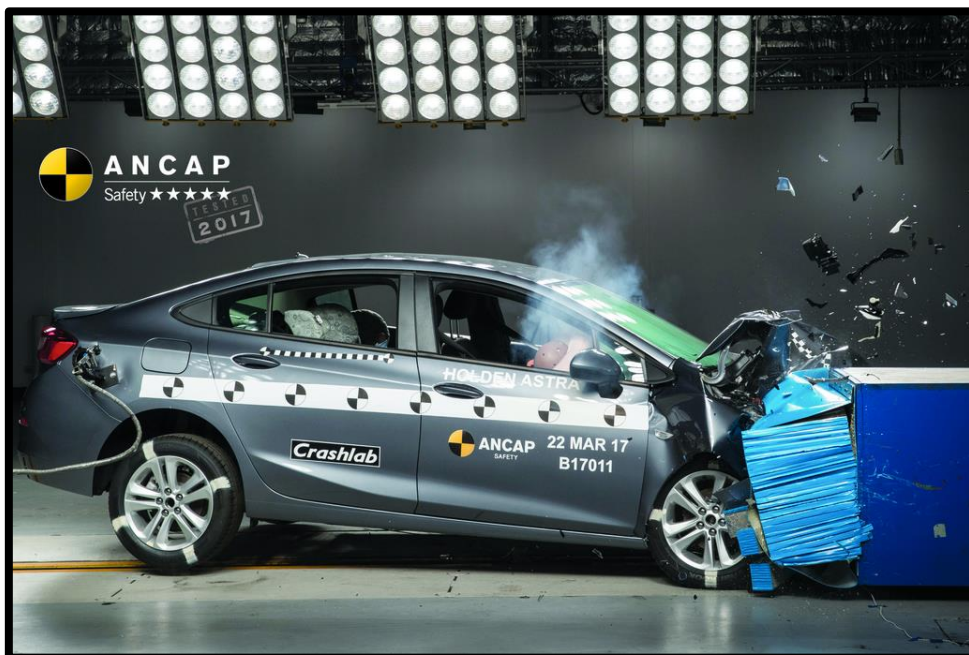
Figure 1 - Holden Astra (May 2017 – onwards) frontal offset test at 64km/h.
